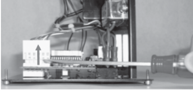
Figure 5: Depicting the Proper Way To Remove Wire Harness Connectors Using a Flathead Screwdriver
