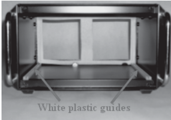
Figure 9: Highlighting the White Plastic Guides On the Bottom of the Case
